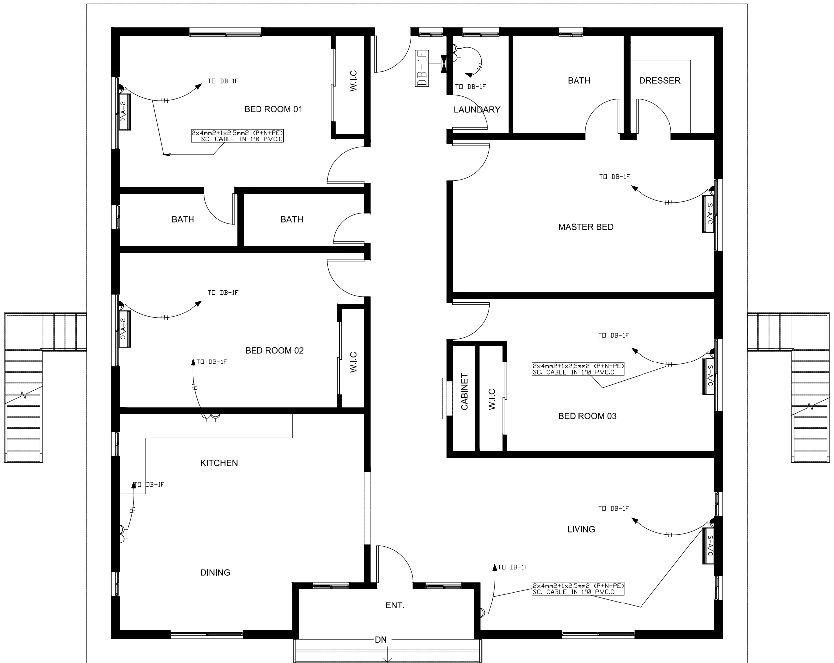
POWER & AC'S LAYOUT FIRST FLOOR
