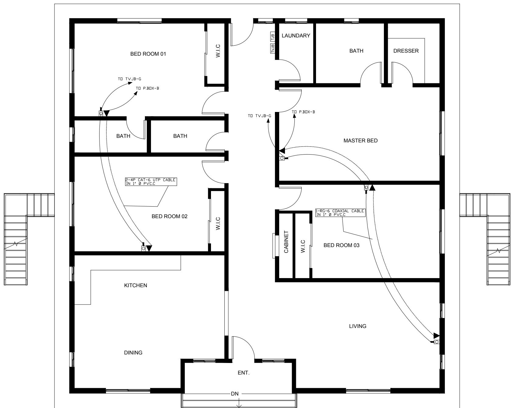
TELEPHONE, TV & DATA CABLE LAYOUT FIRST FLOOR
